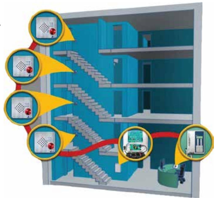
Elevator bays and stairwell landings use Pro-Alert 480 for two-way emergency communications
